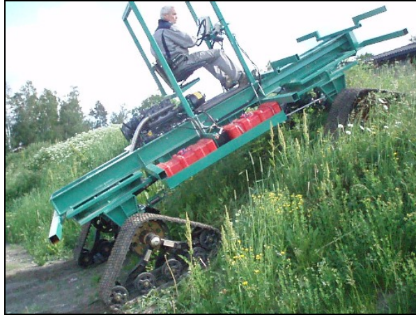
Fig 5 The GT (Getting There) with individual belts. Two tanks can be seen for diesel and PPO. The vehicle use the payload to get equal weight on both axles for best traction.
